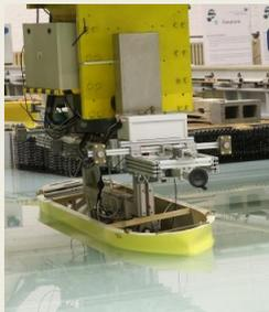
In December 2016, the towing carriage of the towing tank has received a significant upgrade. From now on, it is possible to fully steer a ship model in 4 degrees of freedom (surge, sway, roll and yaw). The first ship model which will run a captive 4 DOF program is the well-known [benchmark container ship KCS](#), newly built at scale 1/52.667. The KCS will be tested at four different under keel clearances, at different constant heel angles and including harmonic roll motion as well.
