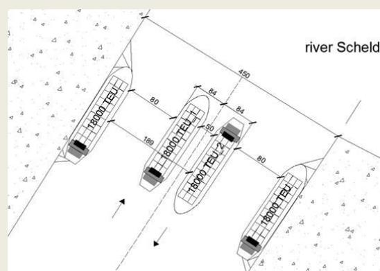
The numerical results were compared with PIANC guidelines with respect to acceptable ship motions and the allowable forces in the mooring lines and fenders. The results of the study, which contain recommendations for passing ships, are being communicated to the river pilots by the [Antwerp Port Authority](#) and generally appear to match the intended speed ranges the pilots have in mind for a safe passage in the given studied situations.
