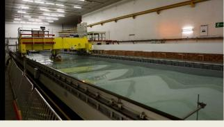
Systematic series of captive model tests have also been carried out in the shallow water towing tank for an ongoing PhD Research project. The main purpose of the research project is to incorporate wave effects into a mathematical ship manoeuvring model. Several researchers have developed such models for manoeuvring in deep water, where the problem can be split up between a
