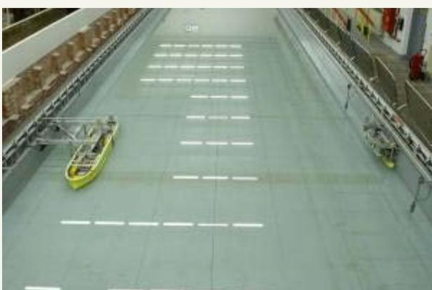
To cope with these questions, a captive model test program is being carried out at the [towing tank for manoeuvres in shallow water](#) for different under keel clearances and dock widths. Four set-ups are tested: the interaction between a passing container vessel and two moored container vessels; the interaction between a passing container vessel and a moored tanker and inland vessel; the interaction between a swinging container vessel and up to two moored
